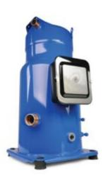
Producer: **Danfoss** Line: **SZ** Cooling capacity [kW]: **20.64** Displacement [m<sup>3</sup>/h]: **37.7** Refrigerant: **R134a, R404A, R407C** Capacity control: **None** Power supply: **400V/3Ph/50Hz**
